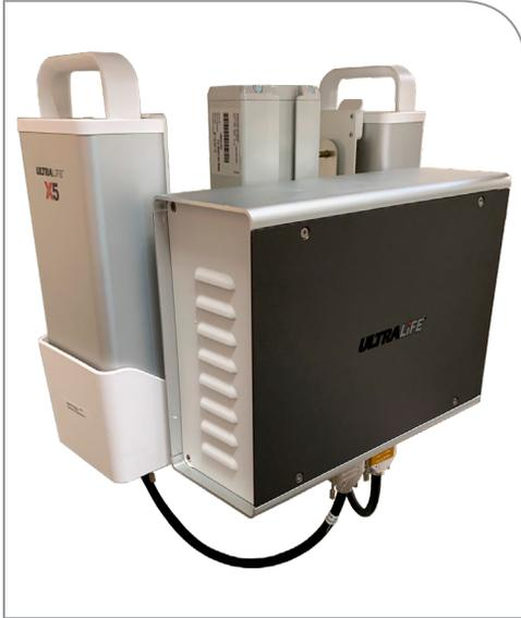
The URS-X5-01 is a revolutionary new power system for medical carts that can be configured to use one or two 276Wh hot swappable batteries, 492Wh embedded U1 batteries or a combination of both. The integrated 72Wh hold-up battery provides 5 minutes of operation during battery swap out operations making the Ultralife URS-X5-01 the most powerful and versatile medial cart power system on the market.
