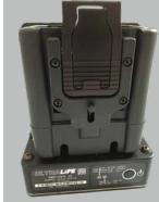
MRC-UVA-V1 is a handheld radio charging solution for vehicle communications. It is compatible with new radios (such as Harris PRC-163, IMBITR. MBITR2, ViaSat PRC-161 and Tactical Network Rover), as well as legacy Harris and Thales radios (plus other radios and devices using the same batteries). It
