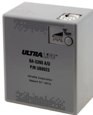
The battery has a single, coulomb counting state of charge indicator that is push button activated. The indicator is comprised of LED display that increases in brightness as the button is held down. This feature allows the user to obtain state of charge information in low-light environments. State of charge information allows the operator to determine if a battery has been used previously and how much original capacity remains.
