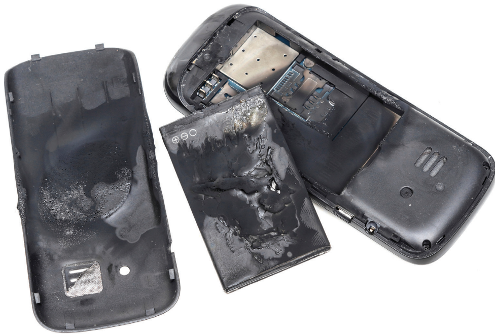
Batteries must not leak, vent, disassemble, rupture or have fire
